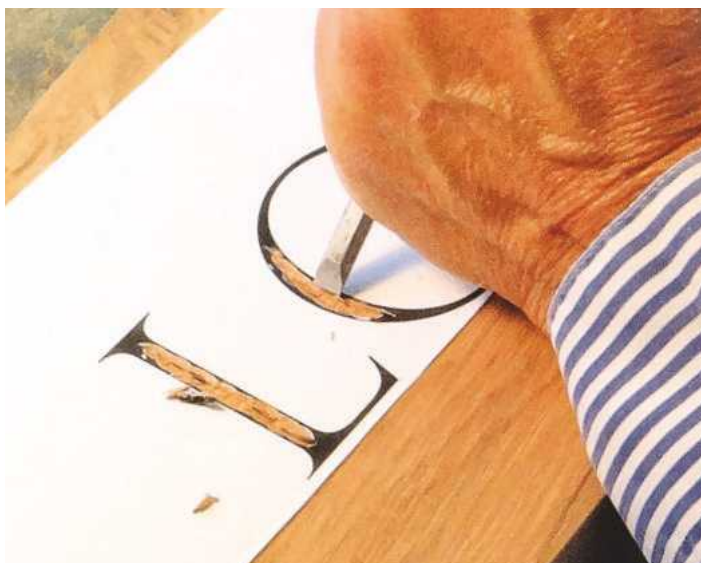
A chisel is necessary for the inside of the O. You might imagine that the O is the hardest letter to carve, but not so. Go round and round, inside and out, maintaining 45° and restraint, and the letter develops by itself. A light touch is needed with the chisel lest it mark the valley. Edward used a wider, flatter gouge to help clean the outer cut
